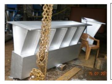
Entry snouts are used as the last guide cum insulation chamber and fixed just prior to the zinc bath.
